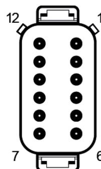
**Please note:** Pins 1 and 5, 2 and 6 must be connected for operation.
